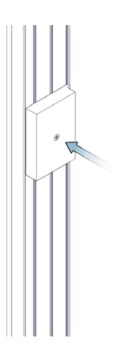
Cut down 5mm frame packers to 72mm (one for each jamb packer)
