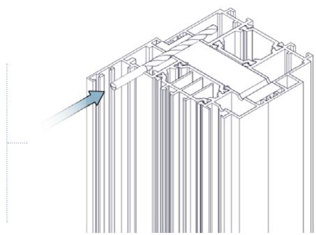
Using supplied screws, fix the window frame to the door jamb, through the jamb packers
