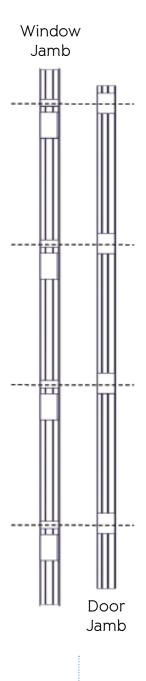
Ensure packers are spaced the same as the frame packers installed on the window frame and fix appropriately
