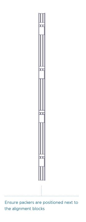
Re-position the jamb packers in the jamb
