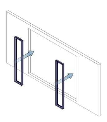
Ensure the remaining aperature is 6mm wider than the overall door set width
