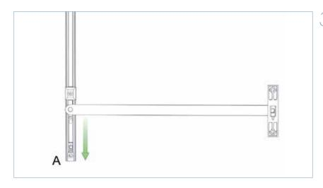
Ensure the slider stop is engaged by placing point (A) against a hard surface and pushing down on the restrictor arm. This will require some force and should result in a click. The restrictor arm should no longer be able to slide up and down the slider housing once this step has been completed.
