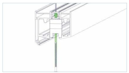
7. Using one of the 5.0 x 45mm screws, secure the middle restrictor block as shown.
