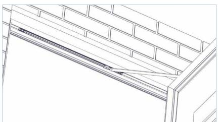
Insert the slider casing into the top track making sure it is still connected to the sash pivot, it should only fit in one position. Then, using a non-permanent method, mark the positions of the four screw holes in the slider casing, then move the slider casing out of the way.
