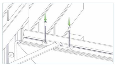
Fit the sash pivot to the top of the door, 60mm from the end of the black polyamide strip on the hinge side using two of the 5.0 x 45mm screws provided. The pivot should be fitted so that it butts up to the edge of the polyamide closest to inside of the door.
