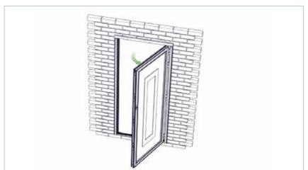
2. Prop the door open to the desired maximum angle.
