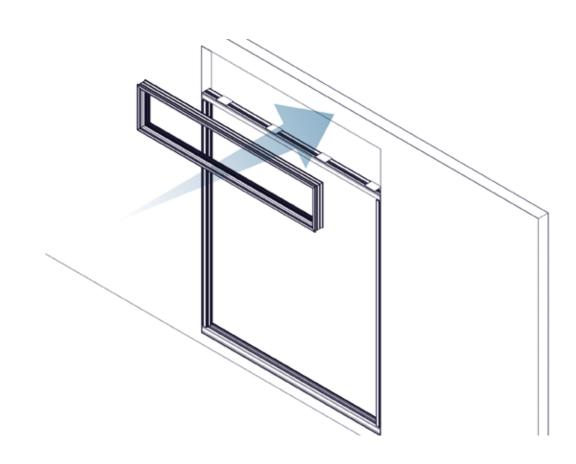
Pre-drill the frame with a 3mm long series drill bit as shown for every alignment block used
